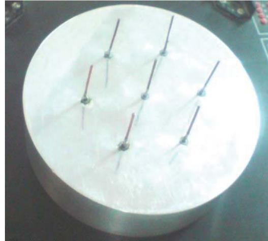
Fig. 4. Designed seven element parasitic switched array antenna.
