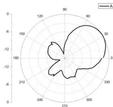
Fig. 8. Anechoic chamber results for  $\phi=30^{\circ}$ .
