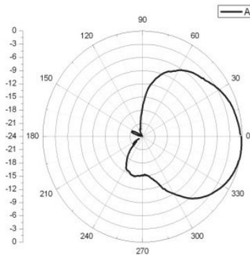
Fig. 7. Anechoic chamber results for  $\phi=0^{\circ}$ .
