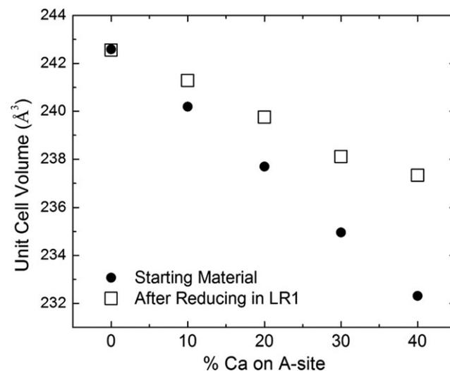
**Fig. 5.** Rietveld refinement of XRD data shows the volume expansion of the perovskite unit cell as a result of both the transformation of Fe<sup>3+</sup> → Fe<sup>4+</sup> and the formation of oxygen vacancies in mass loss region #1 (LR1).
