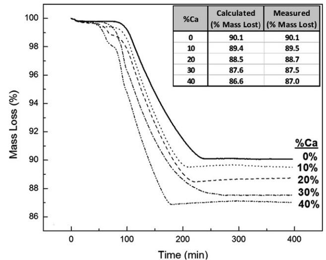
**Fig. 3.** Thermogravimetric data showing the mass loss kinetics to full decomposition in 6%  $\text{H}_2$  at 1100°C. The mass loss was consistent with the formation of CaO,  $\text{La}_2\text{O}_3$ , and metallic Fe, with a maximum deviation of less than 0.5% from theoretical values shown in the inset.
