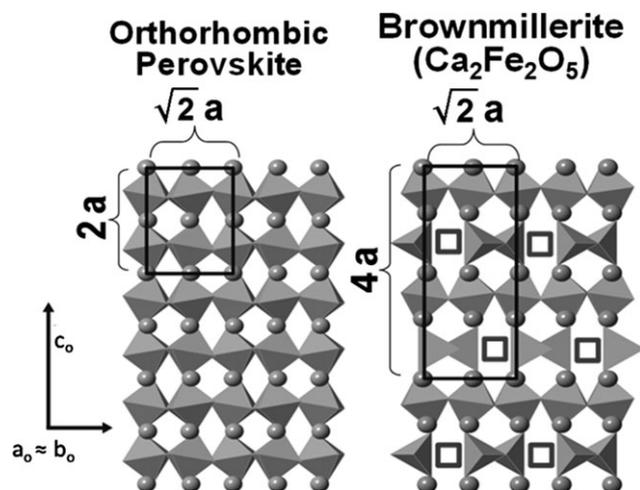
**Fig. 1.** The LCF perovskite structure is composed of large A-site cations, Fe cations located at the center of each octahedra, and oxygen atoms located at the vertices of the octahedra. Ordered oxygen vacancies may form along the [110] direction transforming octahedra to tetrahedra as indicated by the squares in the brownmillerite structure shown above.
