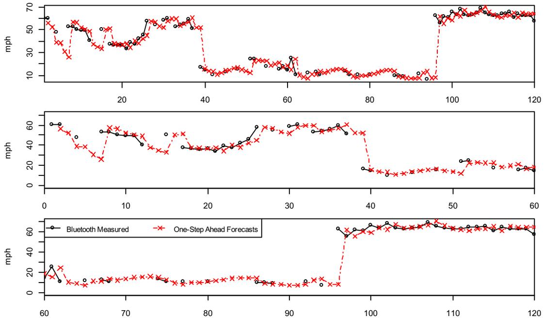
Figure 4. Bluetooth measured one-step-ahead forecasts during incident.
