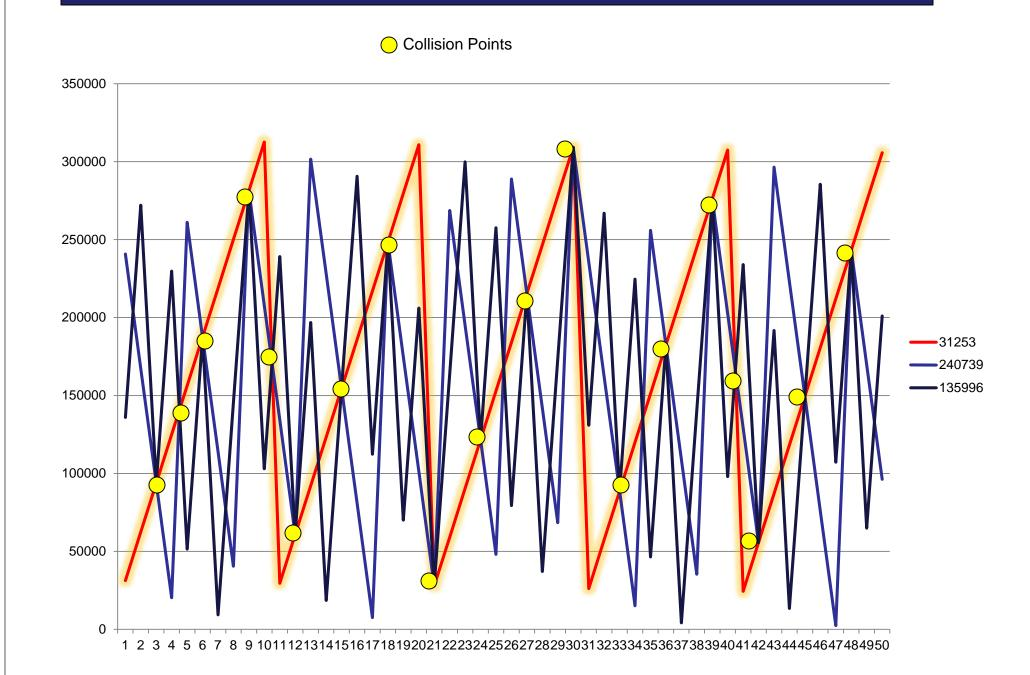
The pattern of the regular protocol is easily identifiable and vulnerable to attack due to its predictability with just a small amount of data collection. There are also several collision points, making it possible for imposter dongles to authenticate.
