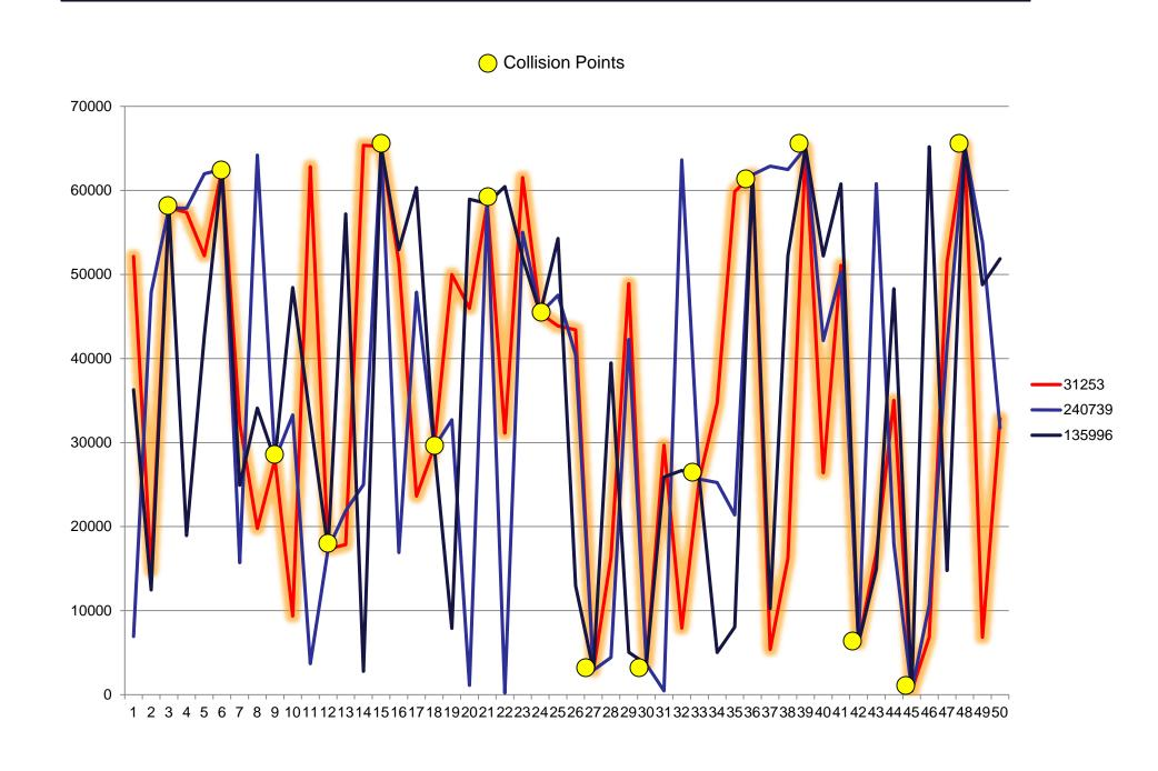
The pattern of 'A' value is disguised by AES encryption of the 'y' value. However, all possible 'A' values converge to the same value where x is equal to a factor of 'n.' This is an algebraic vulnerability of the function that exists with or without hashing any values.
