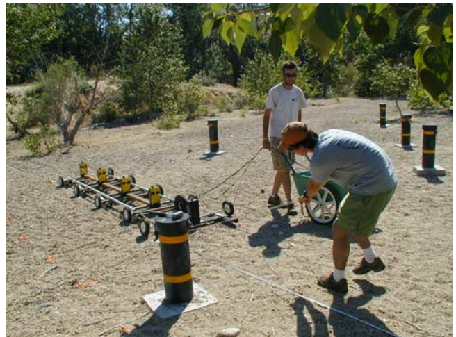
Figure 5. Photograph illustrating the four-receiver acquisition system. The survey was repeated four times with the near offset at 1, 5, 9, and 13 m and 1 m between receivers.
