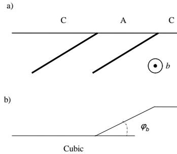
Fig. 2. The *ac* twin found in Fig. 1 (a) after polishing and (b) at a temperature above the martensitic transformation where a double kink appears at the position of the former A domain. The angles are equal and opposite to the angles in Fig. 1.
