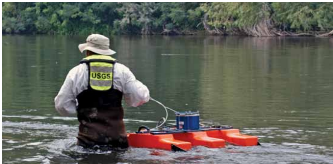
A U.S. Geological Survey hydrologic technician measuring streamflow
