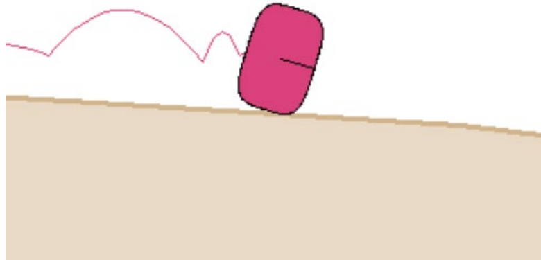
Figure 4.3: Rock Shape (Super ellipse ^4 2:3 ) in RocFall2
