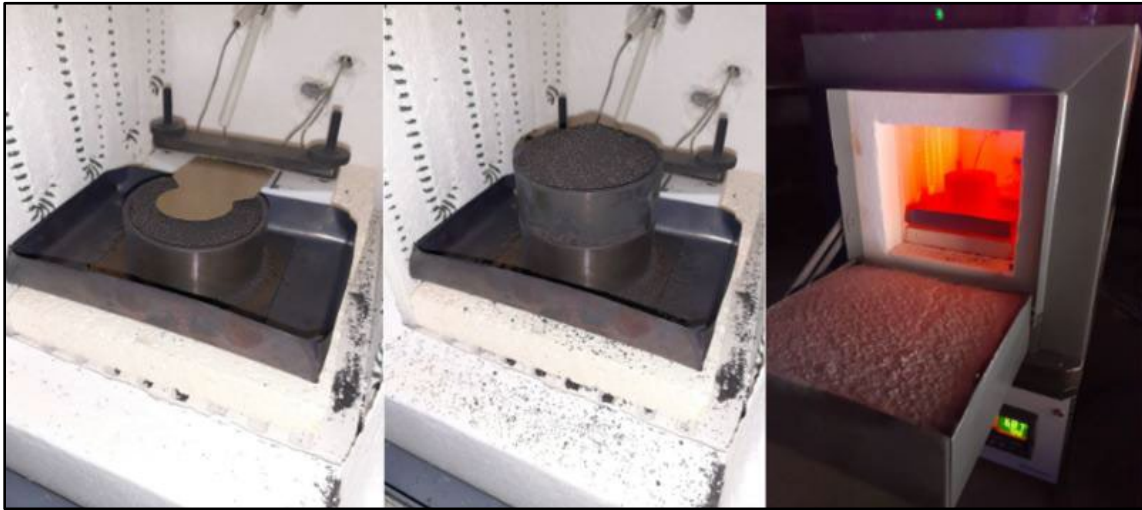
Figure 2.5 Process of loading the stainless-steel testing chamber with particles and embedding an F1 4901 Mica sensor. The sensor is connected to the Hot Disk TPS 2500 S via a PEEK High-Temperature cable. The apparatus is housed within a Thermolyne FB1415 Benchtop Muffle Furnace for high-temperature testing.
