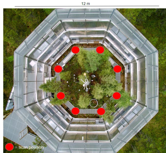
Figure 3.2. Nadir view of a chambered plot at the SPRUCE site. Red circles indicate TLS scan position locations.
