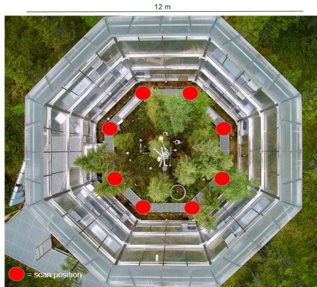
Figure 2.2. Nadir view of a chambered plot at the SPRUCE site. Red circles indicate TLS scan position locations.
