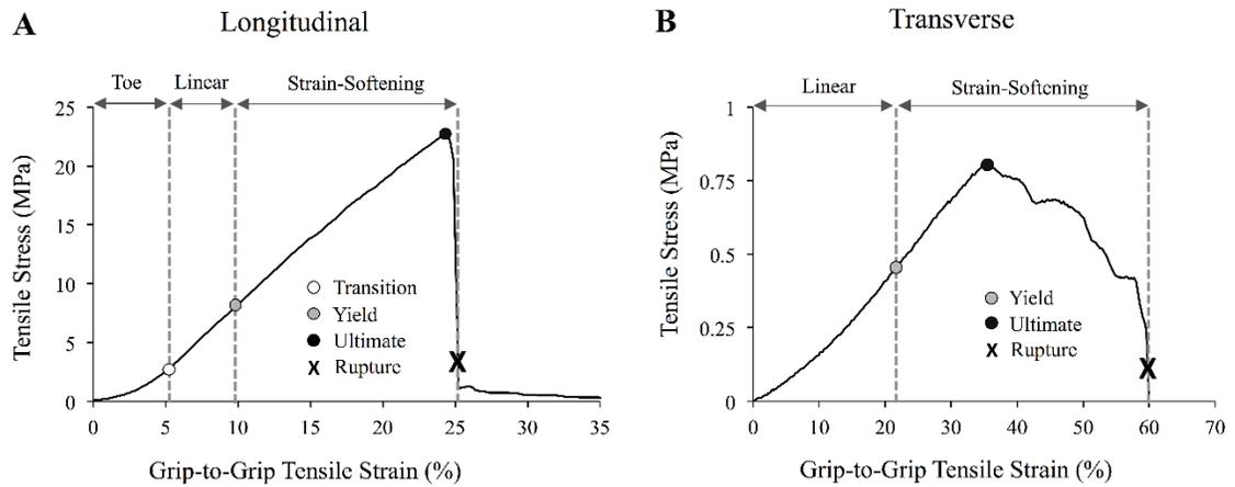
**Figure 7: Representative stress–strain curve for a A) longitudinal and B) transverse specimen with marked points of interest (transition, yield, ultimate, rupture). Grip-to-grip tensile strain was measured as the grip displacement divided by the grip-to-grip reference length.**
