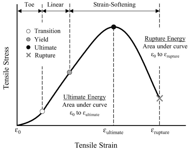
**Figure 12: Representative tensile stress-strain curve of soft tissue with marked points of interest (transition, yield, ultimate, and rupture), as well as different measures of strain energy density.**
