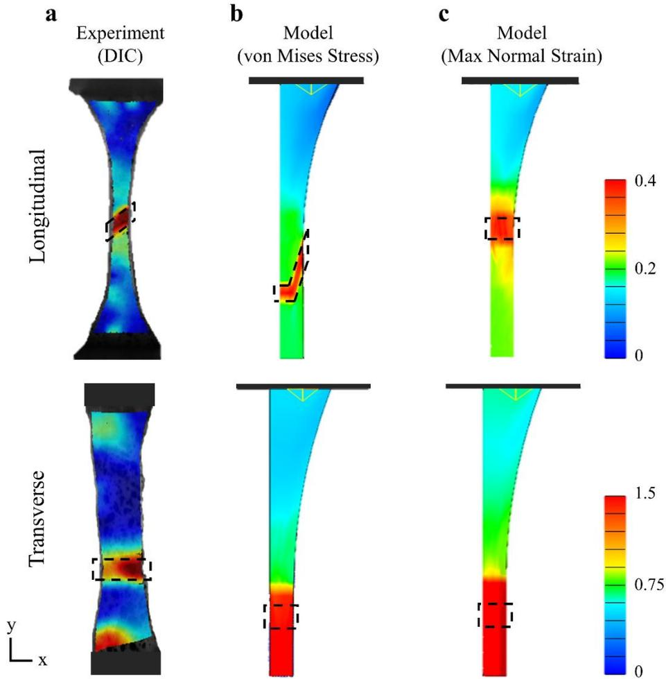
**Figure 22: Normal strains ( $E_{yy}$ ) from experiments and FE models for longitudinal and transverse specimens. A) The experimental tear pattern and strains in the tear region (ROI) measured with DIC were compared to model predictions using b) von Mises stress damage criteria, and c) maximum normal strain damage criteria. ROI are shown above by the dashed black box.**
