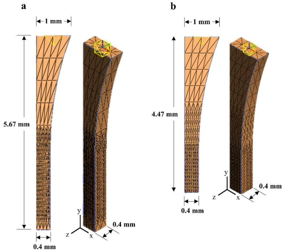
**Figure 19: Coupon dimensions and mesh for all a) longitudinal and b) transverse models.**
