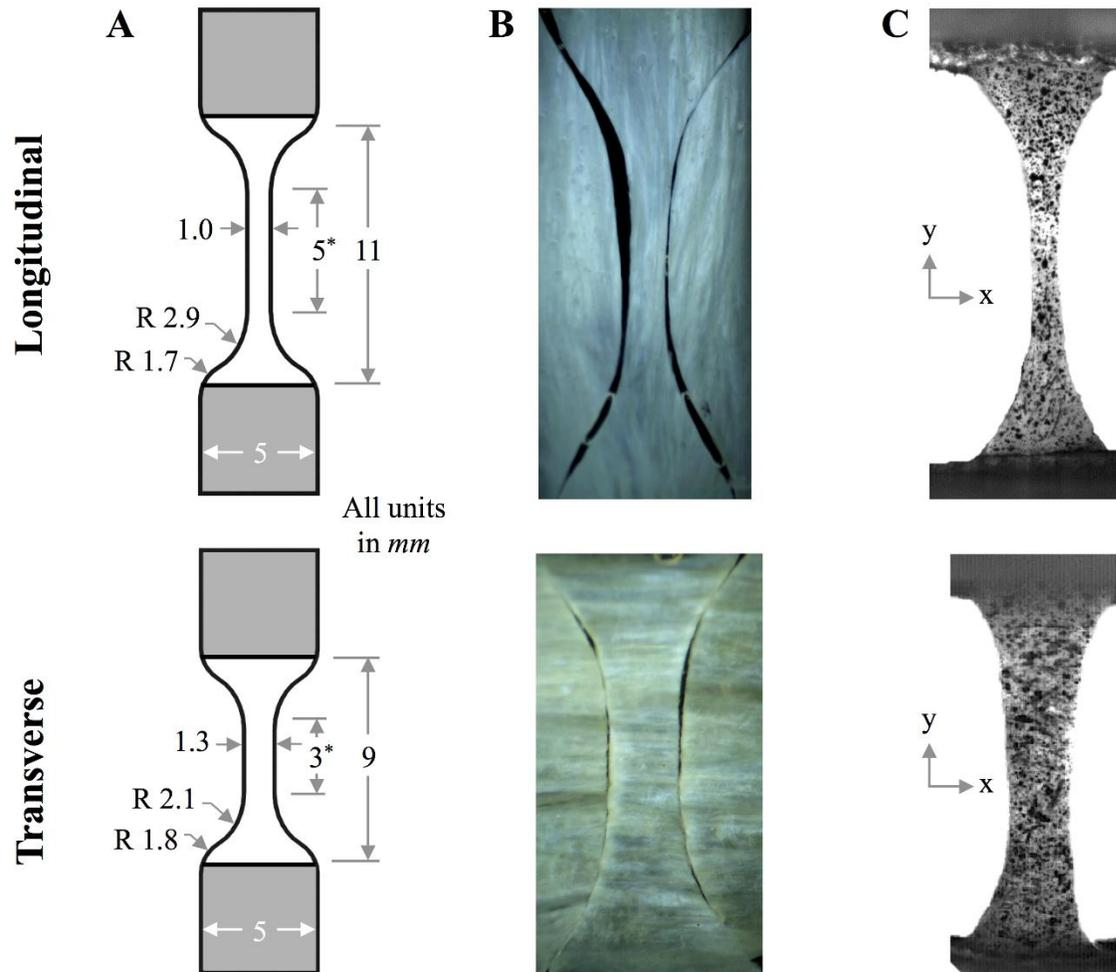
**Figure 4: Longitudinal and transverse tensile specimens from human meniscus. A) Dimensions of dumbbell coupons in mm (gray = region being gripped, \* = gauge section). B) Light microscopy of tissue coupons captured the visible fiber orientation prior to mechanical testing. The mean fiber orientation was quantified using FiberFit software. C) Specimens with a sprayed speckle pattern for DIC analysis.**
