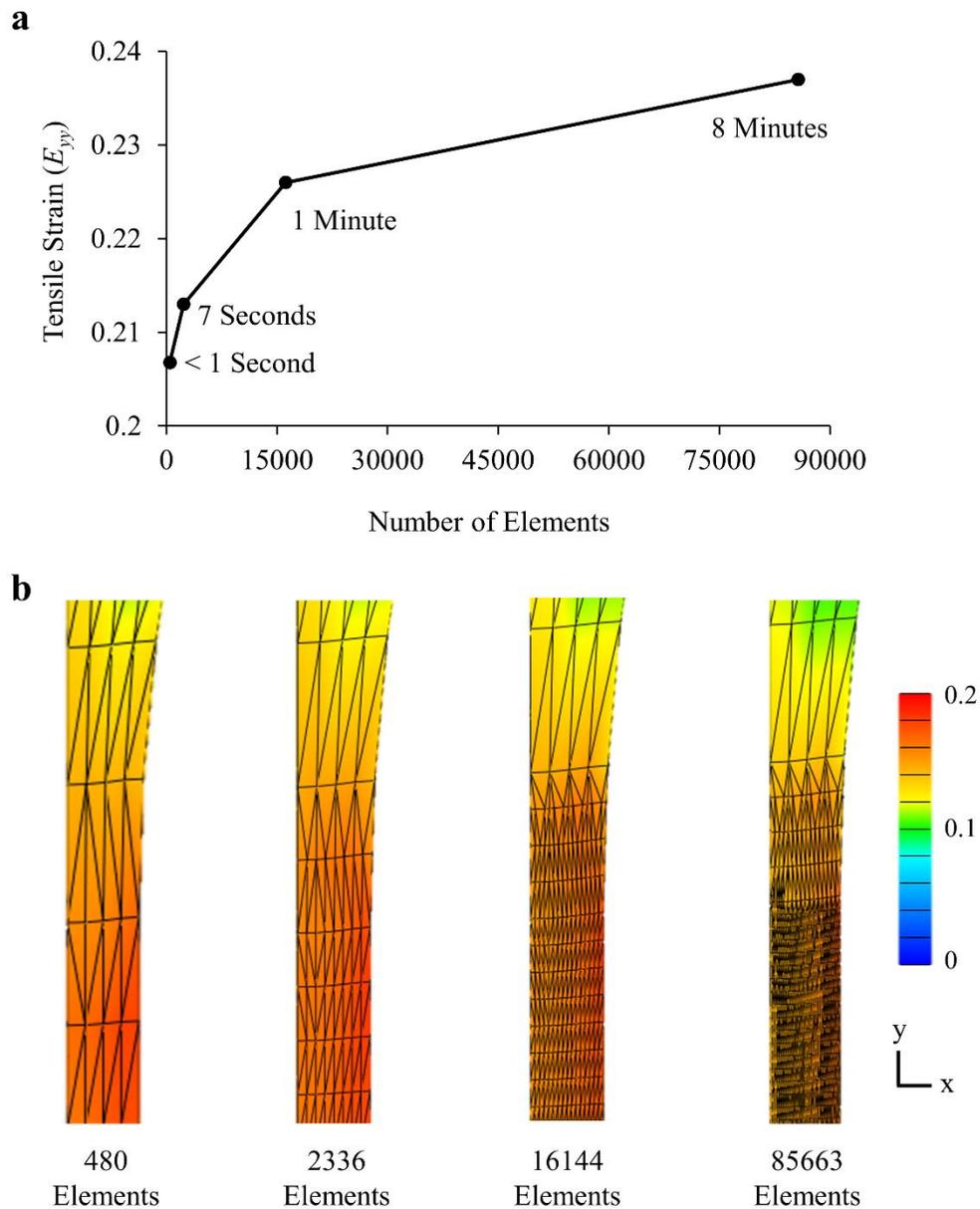
**Figure 20: Mesh convergence study. a) Increasing mesh size resulted in longer run times and greater tensile strain ( $E_{yy}$ ) inside the tear region that gradually plateaued. b) Strain maps ( $E_{yy}$ ) of different mesh sizes. This study used 16,144 elements.**
