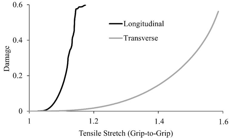
**Figure 21: Maximum damage in the tear region of two representative specimens.**
