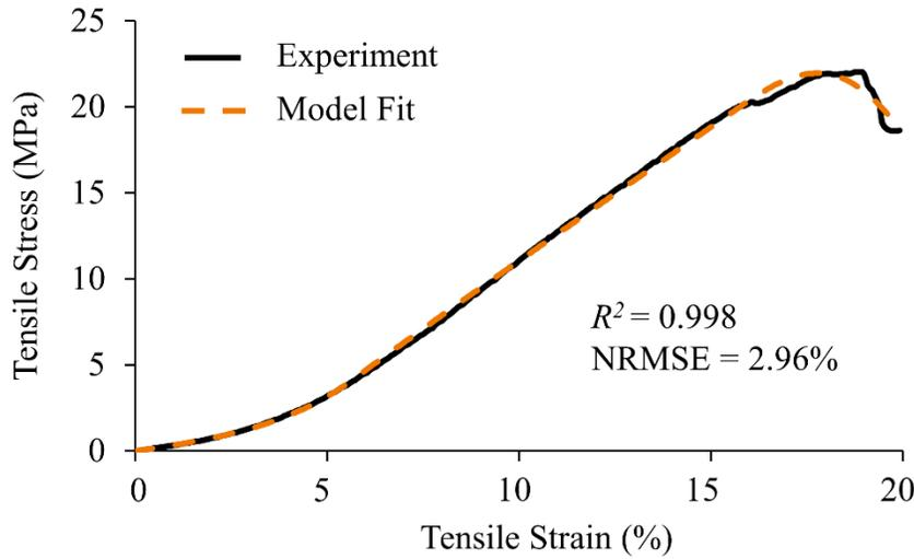
**Figure 14: The hyperelastic-damage model gave excellent fits to the experimental data.**
