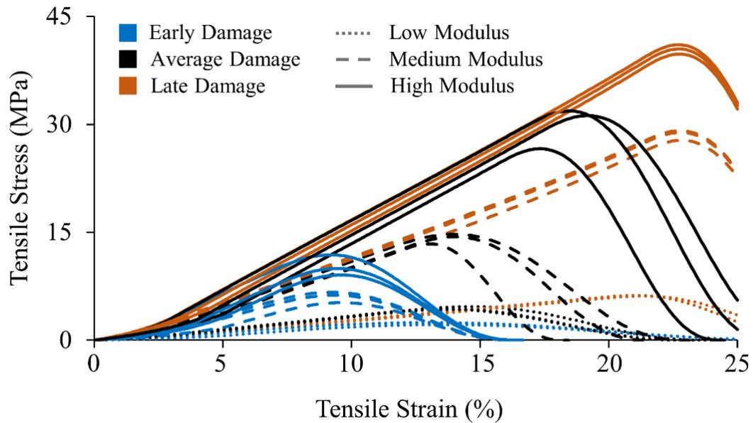
**Figure 15: Model generated stress-strain curves using three different settings for transition strain, linear modulus, and damage onset, resulting in 27 unique curves with known transition strains.**
