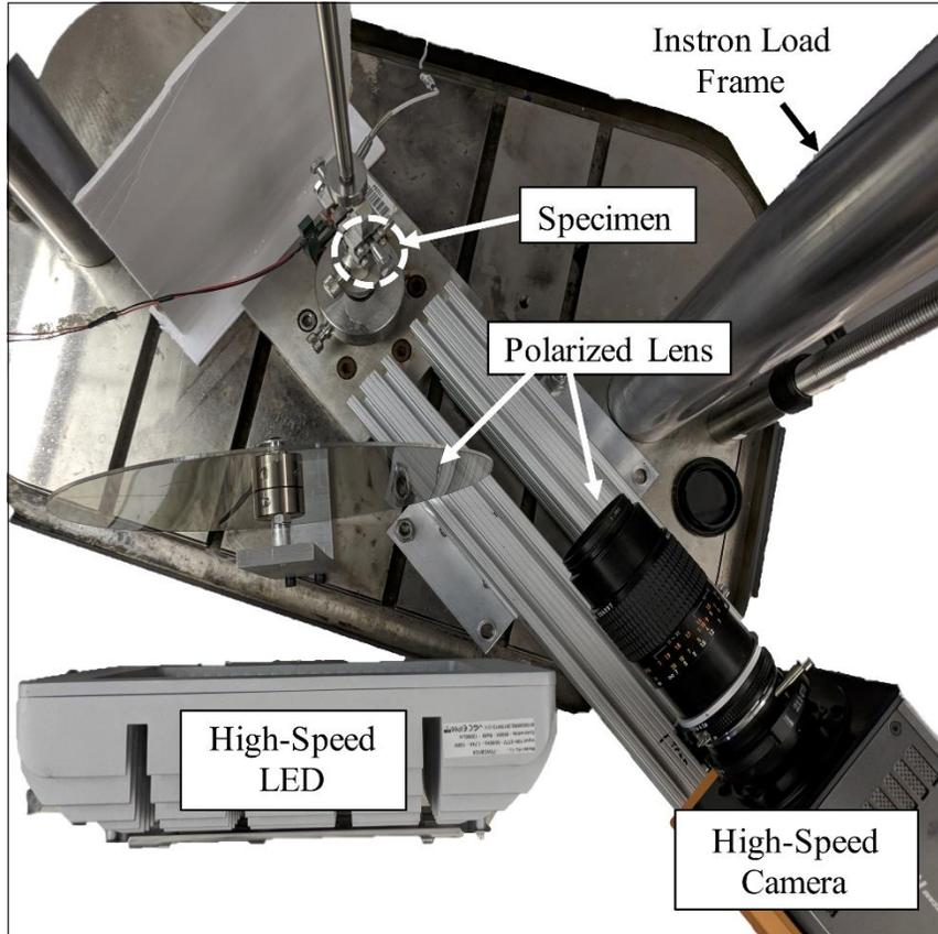
**Figure 5: Top view of the tensile test setup for high-speed measurement of full-field strain. In order to minimize glare on the specimen surface, two polarized lenses were positioned between the LED and camera with polarization angles in  $90^\circ$  opposition to each other.**
