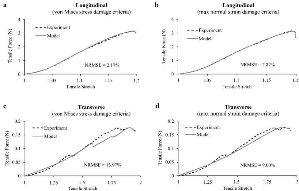
**Figure 23: Representative model fits to experimental grip-to-grip force–displacement curves (we converted grip displacement to tensile stretch). (a) When modeling the fiber response (longitudinal), von Mises stress damage criterion had better fits compared to the (b) maximum normal strain damage criterion. (c) However, von Mises stress damage criterion had slightly poorer quality of fits compared to (d) maximum normal strain damage criterion when modeling the ground substance (transverse).**
