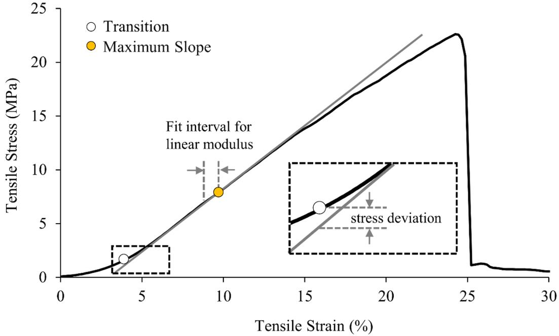
**Figure 13 Graphical depiction of the method used to determine the transition point. The transition point is determined from the deviation between the stress-strain curve and the linear fit to the linear region below the maximum slope. In this study, the fit interval was 1% strain.**
