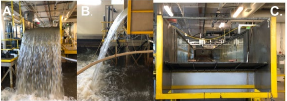
Figure 2.1. A front view [A], side view [B], and main channel view [C] of the Streamlab Flume plunge-pool.
