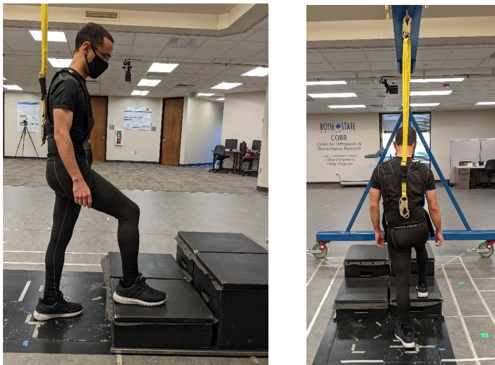
Figure 3.1 Overhead gantry and safety harness used during stair negotiation
