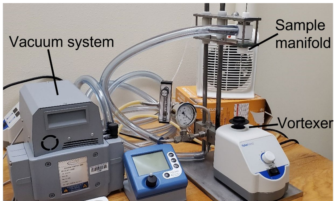
Figure 9 Custom Set Up of the Rapid Solvent Exchange Method.
