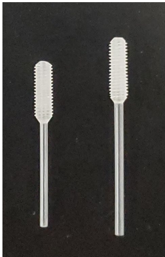
Figure 13 Gas-permeable methylpentene polymer (TPX) capillary used for EPR measurements; 0.8 mm (left) and 1.0 mm (right).
