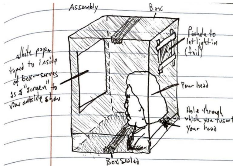
**Figure 8 Student Drawing of a Pinhole Camera**
