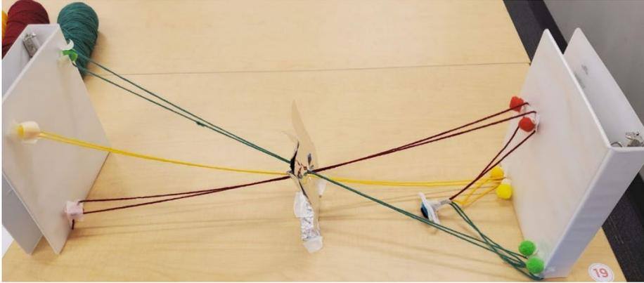
**Figure 12 Photo of Student's Model of Blurriness in a Pinhole Camera**
