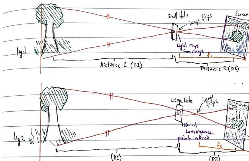
**Figure 9 Student Drawing of How Blurry Image is Created in Pinhole Camera**
