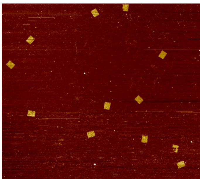
Figure 2S.3. Larger field of view image of several large origami rectangles synthesized using pScaf-11054.1.
