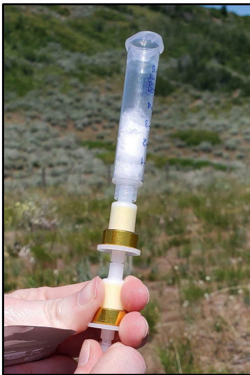
Figure 2 Ambient air collection apparatus. Two DNPH-silica cartridges are attached in series to a Luer lock syringe loaded with KI and CaCl 2 . The first DNPH-silica cartridge in series, A, is placed above the second, B.
