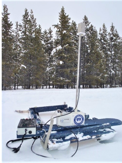
Figure 1.2: The SMP mounted on a sled at the West Yellowstone airfield during the NATC campaign. The SMP was developed and designed by Dr. Martin Schneebeli (SLF) and Dr. Jerome Johnson (CRREL) in the mid-1990s. The pictured sled was designed and built by Dr. Matthew Sturm (CRREL).
