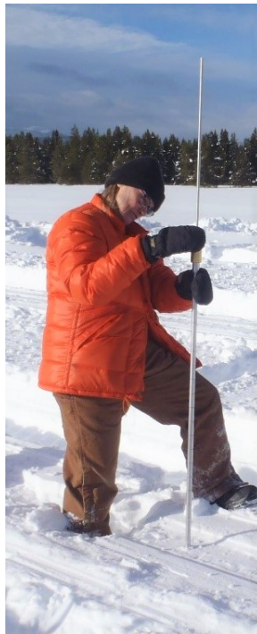
Figure 1.4: CRREL's Dr. Sally Shoop using the ram to measure the hardness of a vehicle belly drag after a coast-down test at NATC.
