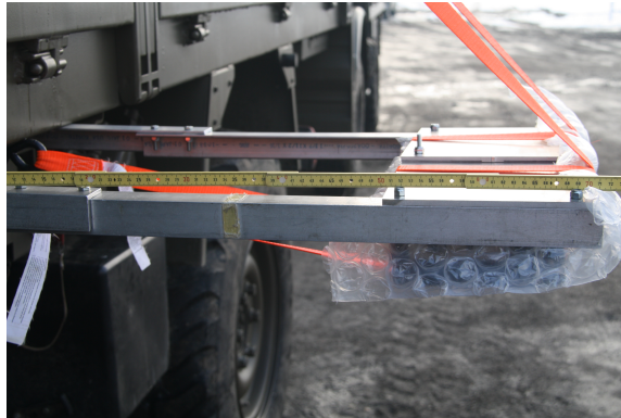
Figure 4.19: 900 MHz GPR antenna mounted on the Mercedes Unimog U 4000. The GPR was operated from the vehicle. Distances were marked in the GPR trace header every 50 m using a GPS odometer. Changes in the ground surface were also marked.
