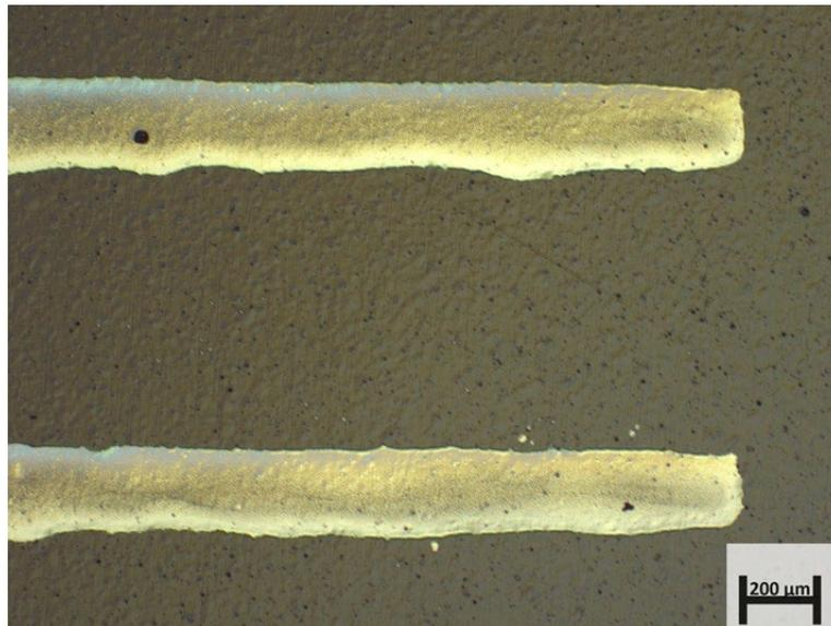
**Figure 11.** Typical microscope image of two print lines.
