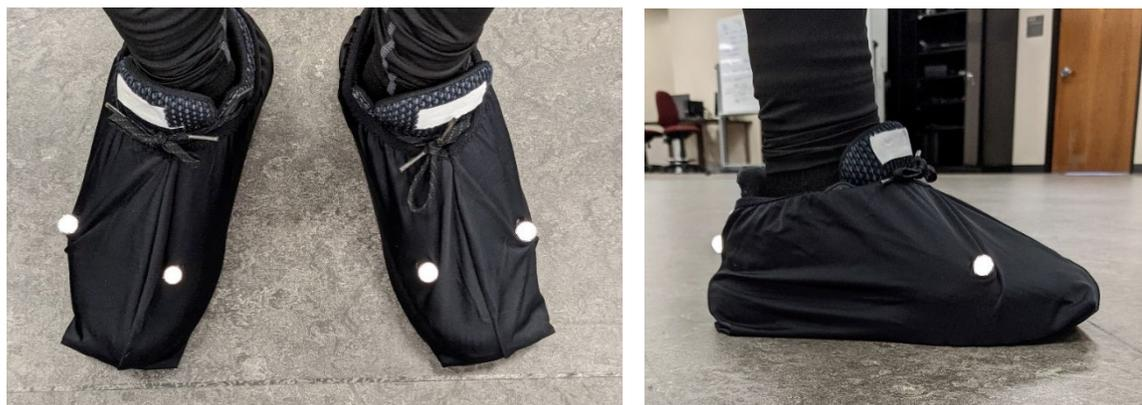
**Figure 3.4** Slick booties outfitted over participant shoes with holes for marker visibility during slick surface stair negotiation
