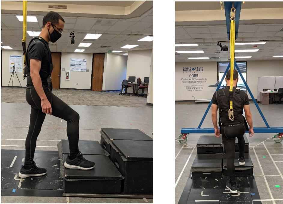
**Figure 3.1** Weight supporting gantry used for stair ascent and stair descent task
