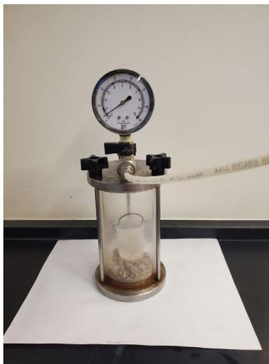
**Figure 2. 5. Photograph showing the rapid carbonate analyser used in this research.**
