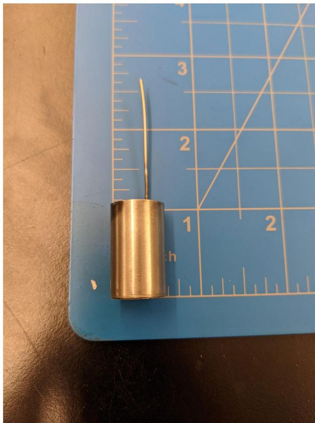
**Figure 10** Zr23 surface polished prior to high temperature EIS run.
