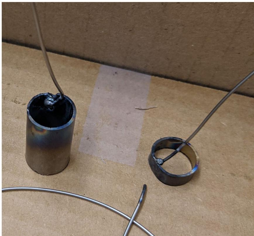
**Figure 12** Zr24 (right) after TIG welding process.
