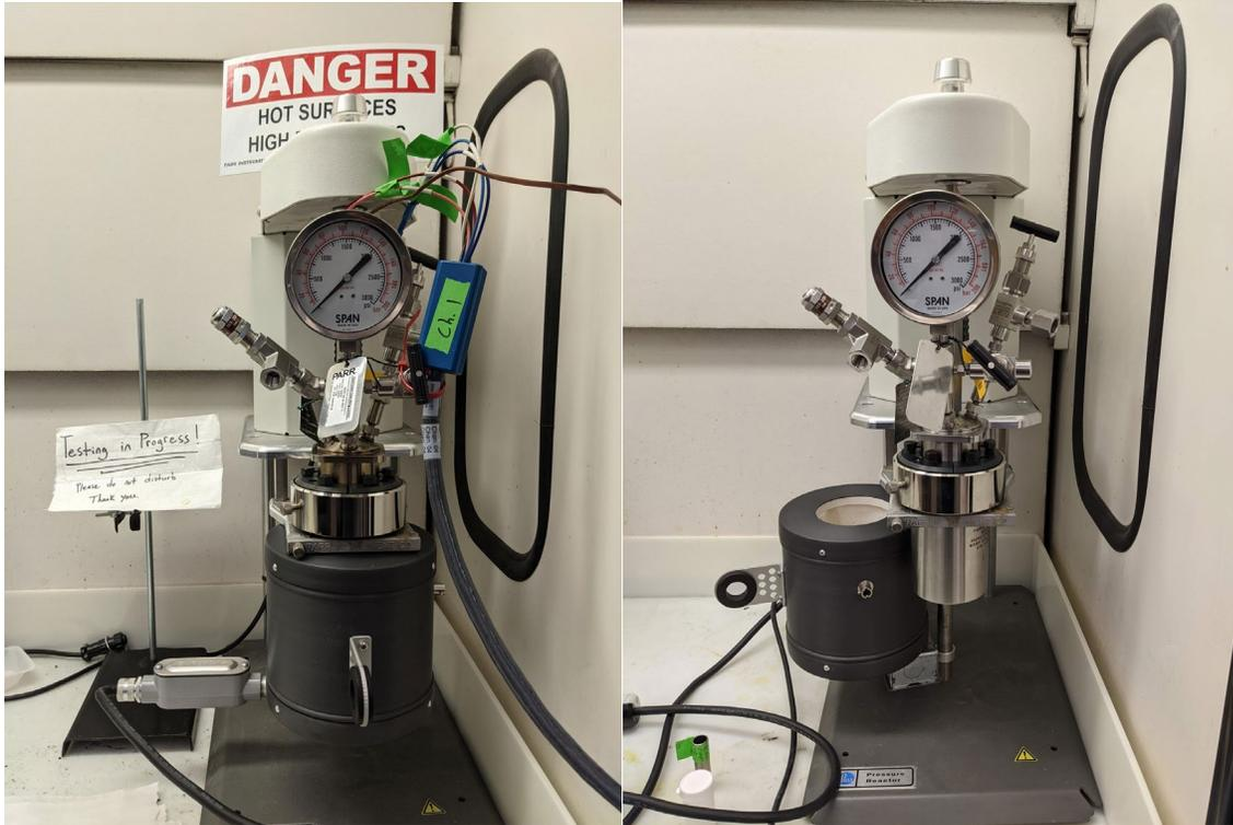
**Figure 8 Hydrothermal reactor connected to potentiostat for impedance data acquisition (left) and before testing (right).**
