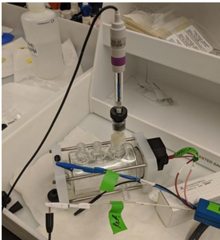
**Figure 6** Experimental setup for room temperature EIS testing.
