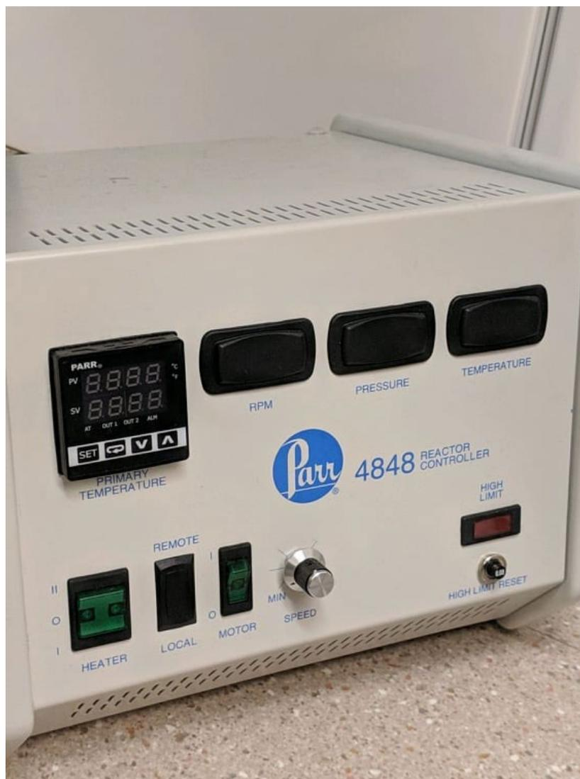
**Figure 7** Reactor controller used in hydrothermal reactor tests.
