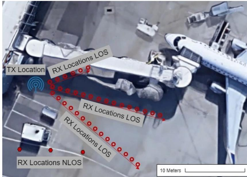
**Figure 3.5:** Map of tarmac at Boise Airport, showing transmitter and receiver designated by dotted lines.
