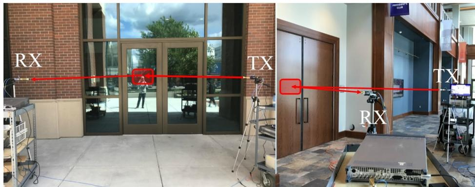
Figure C.4: Pictures of the 81 GHz reflection measurement for outdoor tinted glass (left) and indoor wooden door (right) at AFC. Both TX and RX antennas were bore-sighted on a material with an incident angle indicated by a red box.
