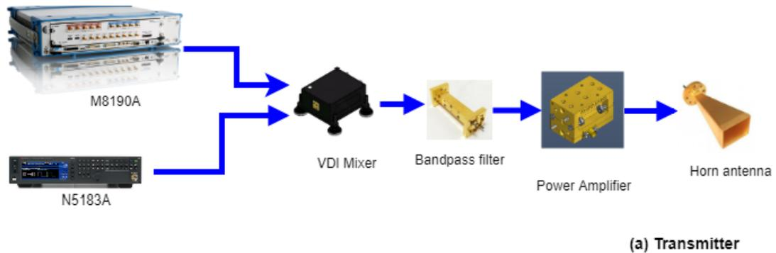
**Figure 3.1: Transmitter setup**
