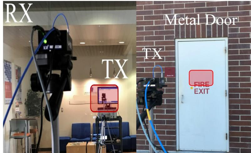
Figure C.3: Pictures of the 73 GHz penetration measurement for indoor clear glass wall (left) at NB and outdoor metal door (right) at MEC. Both TX and RX antennas were bore-sighted on a material indicated by a red box.
