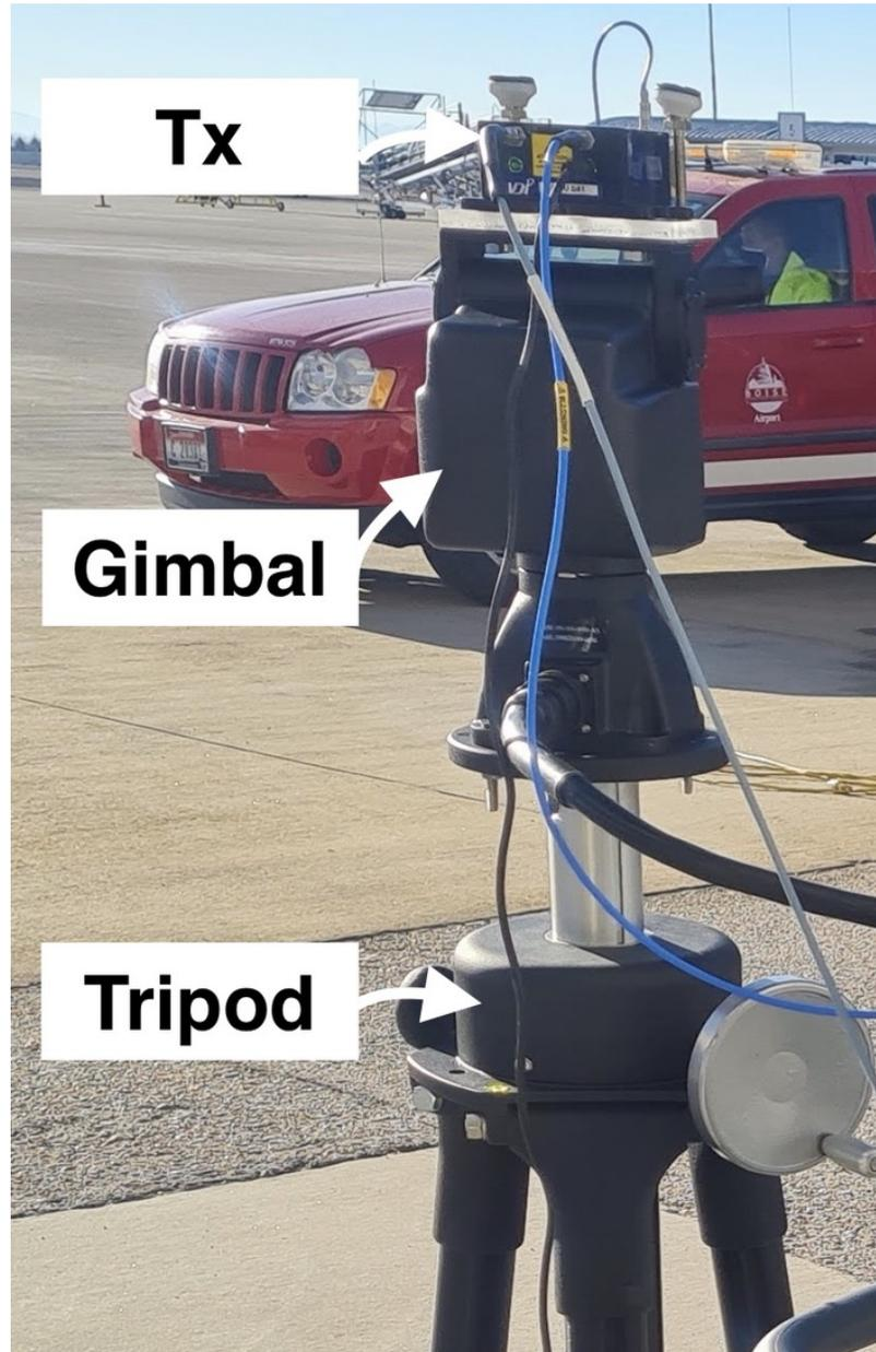
**Figure 4.1: TX gimbal module with gimbal attached to TX antenna and tripod**
