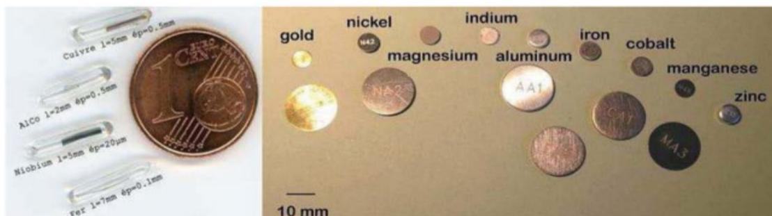
**Figure 1.10** From *Unruh, T. et al*, Representative current state-of-the-art activation wires and foils
