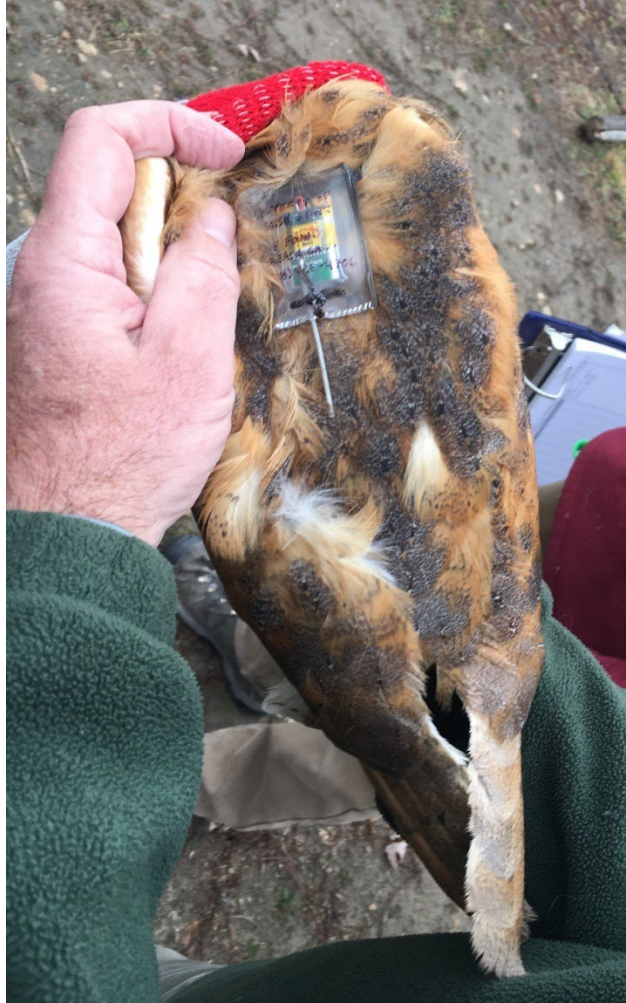
Figure 1.2 A backpack containing a GiPSy-5® data logger attached to an adult female Barn Owl near Homedale, Idaho, USA.
