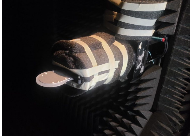
Figure 6.10. Fabricated antenna setup in an anechoic chamber
