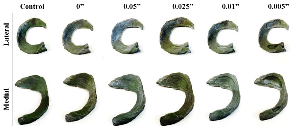
Figure 32. Complex Surrogate Model showing 3D printed meniscus replicas at varying defect depths for both the lateral and medial meniscus
