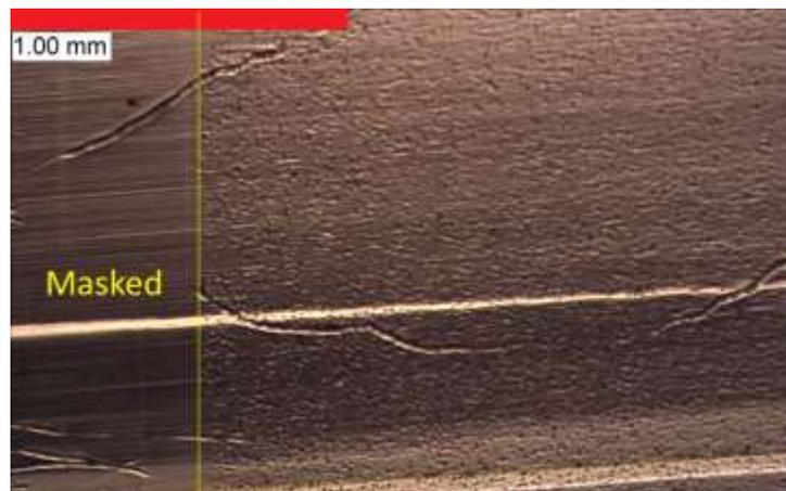
**Figure A-5:** Optical micrograph of a sample at the masking following 15psi peening for 10-second duration. The surface scratches appear to be deeper than the damaged layer.
