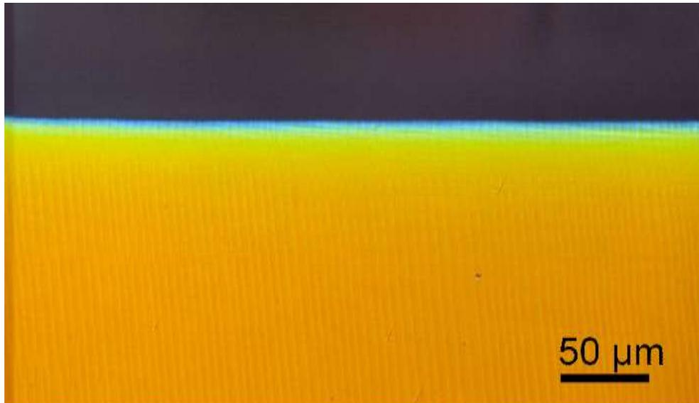
**Figure A-11: The fine twin lamellar structure that is caused by the micropeening surface treatment process. This is taken on the top view after cycling the element 500,000 times in MSM pump manner and following polishing to reveal the twin density.**
