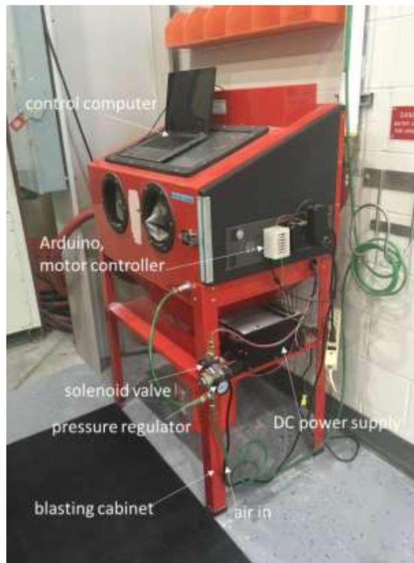
**Figure A-1:** The micropeening apparatus is located within a sandblasting cabinet.
