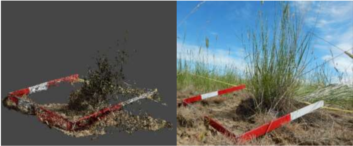
Figure 3.5 SfM point cloud (left) derived from corresponding photo (right) used in reconstruction.
