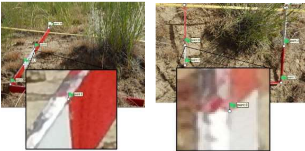
Figure 3.9 An example of marker/point 8 used in image alignment in two slightly different locations on the frame. This error will cause error in the point cloud reconstruction.
