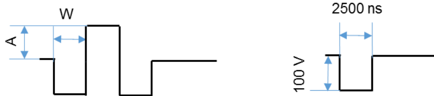
Figure 19 Square wave with amplitude ( A ) and pulse width ( W ). Example of impulse voltage used for experiments pictured right.
