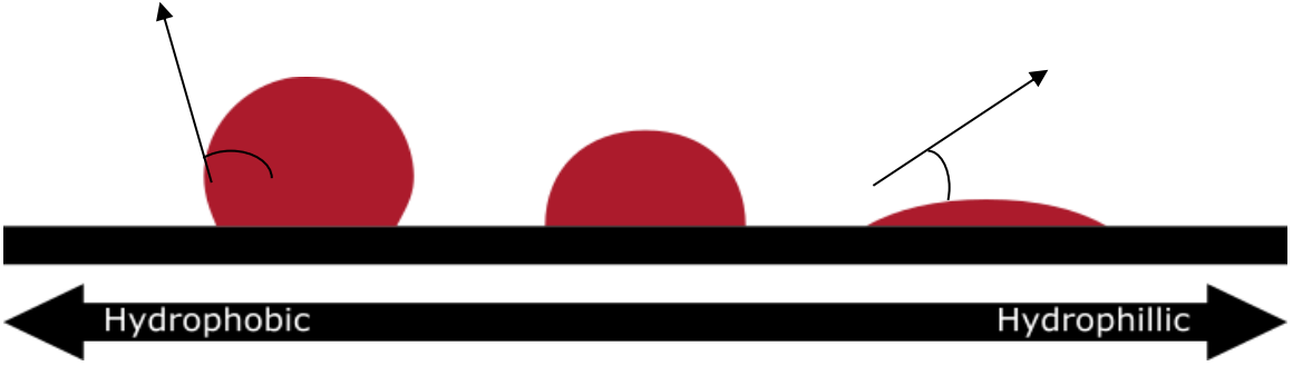
Figure 3.7 Various contact angles [72]
