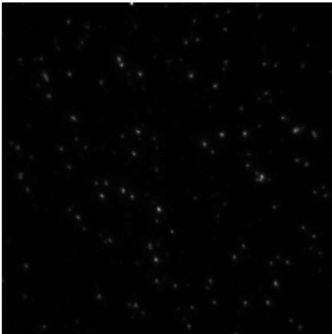
Figure 2.8: Raw image capture of diIC2(5) phosphoramidite dipole emission patterns. Image dimensions are 55 \times 55 \mu\text{m}^2 with a 512 \times 512 pixel ROI and a defocus = 200 nm. The image also contains defocused AuNPs.
