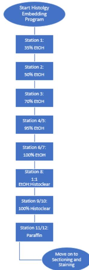
**Figure 4** Flowchart highlighting the steps in dehydration
