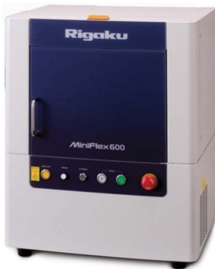
Figure 22 Rigaku Miniflex 600 bench-top X-ray diffractometer. The tool has a 600 W generator with copper source and is capable of a 2\theta scan range of +2 to +145 °. It is capable of very quick scans because of the One-dimensional D/teX Ultrahigh-speed detector. From the Boise State Center for Materials Characterization at Boise State University [38].
