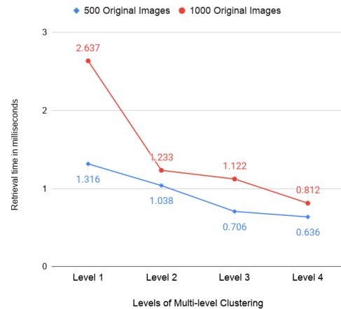
Figure 5.13: Average retrieval time per query at different levels of multi-level clustering with Compression Factor of 64, threshold at 10% and branching factor of 2
