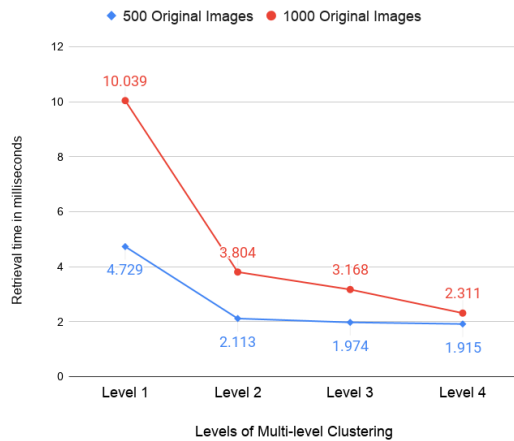
Figure 5.12: Average retrieval time per query at different levels of multi-level clustering with Compression Factor of 16, threshold at 10% and branching factor of 2
