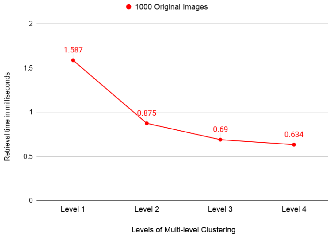
Figure 5.14: Retrieval time per query at different levels of multilevel clustering with Compression Factor of 128, threshold at 10% and branching factor of 2
