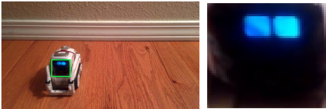
Figure 3.2: Taken from [27]: Example of face tracking and the corresponding extracted face frame.
