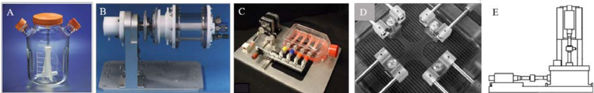
Figure 2 Types of tissue engineering bioreactors. A) Spinner flask, B) Rotating vessel, C) Uniaxial, D) Equibiaxial, and E) Biaxial bioreactor systems.
