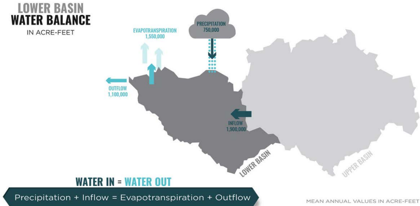
Figure 3. Above shows the mass water balance of the Lower Boise River Basin. The graphic and data come from Boise State University’s Treasure Valley Water Atlas.
