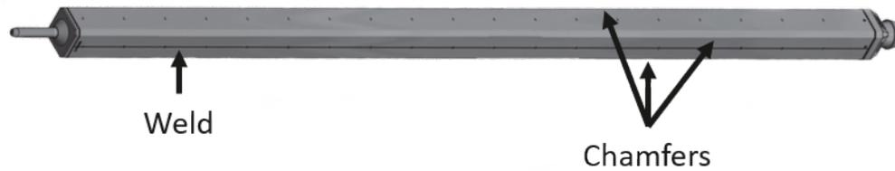
**Figure 1.1: Rendering of the fuel cladding assembly to be used in the TREAT facility.**
