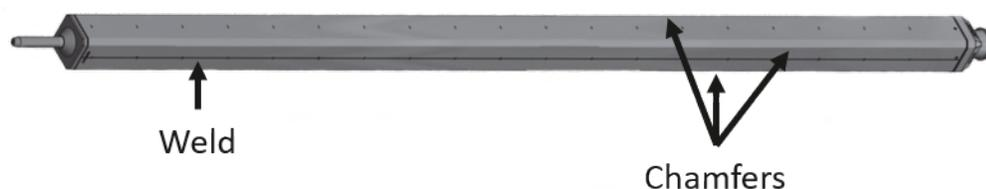
**Figure 3.1: Rendering of TREAT's unique fuel cladding assembly, which includes chamfered corners and welded end caps.**
