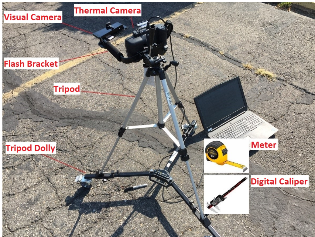
Figure 3- 3. Mobile thermography testing setup
