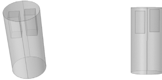
Figure 2- 7. Defects location in the software model
