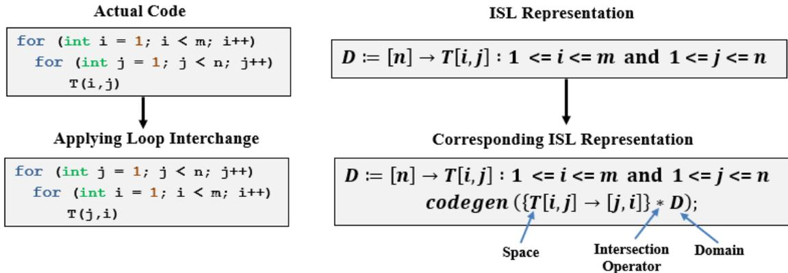
Figure 2.5: An illustration of loop interchange using ISCC.
