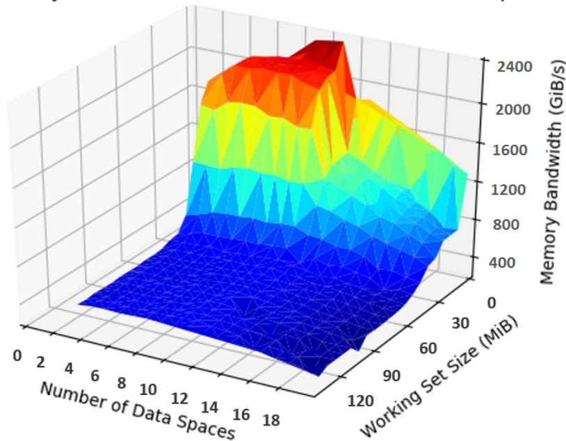
Figure 4.5: An experiment to identify the number of data streams fetching simultaneously that gives optimal performance on parallel execution with 28 threads.
