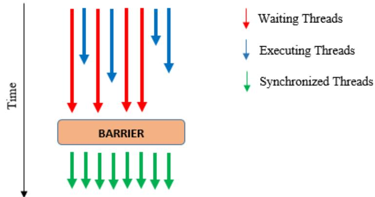
Figure 4.2: Illustration of barriers in multithreaded programming.
