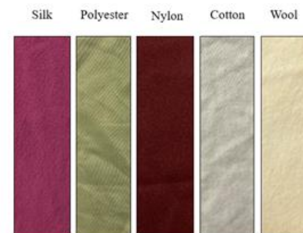
Figure 1. Illustration of the fabric materials evaluated in the study. Each sample was 20cm long and 5cm wide.
