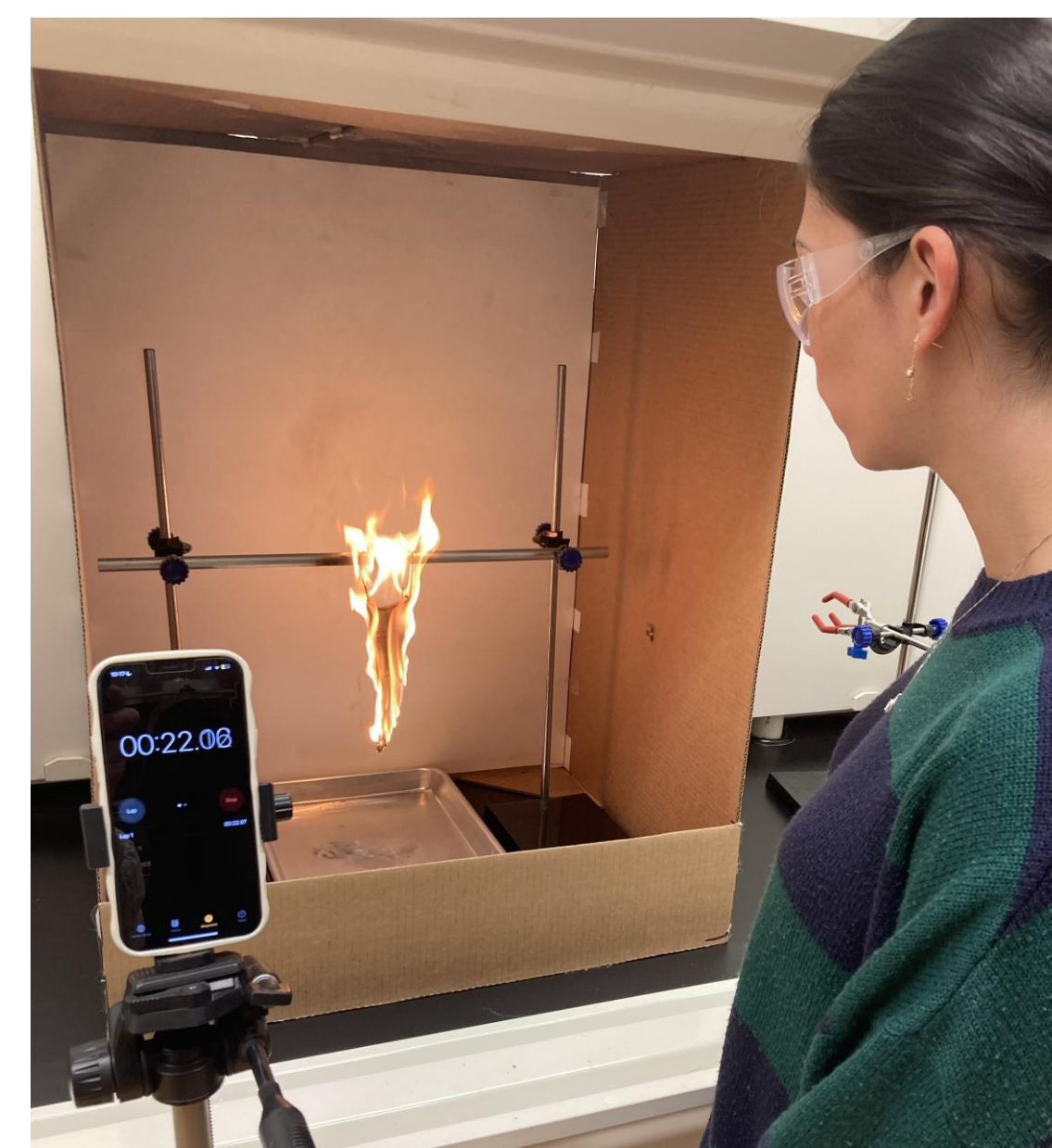
Figure 2. Illustration of a fabric sample burning inside the fume hood and the combustion time being recorded.
