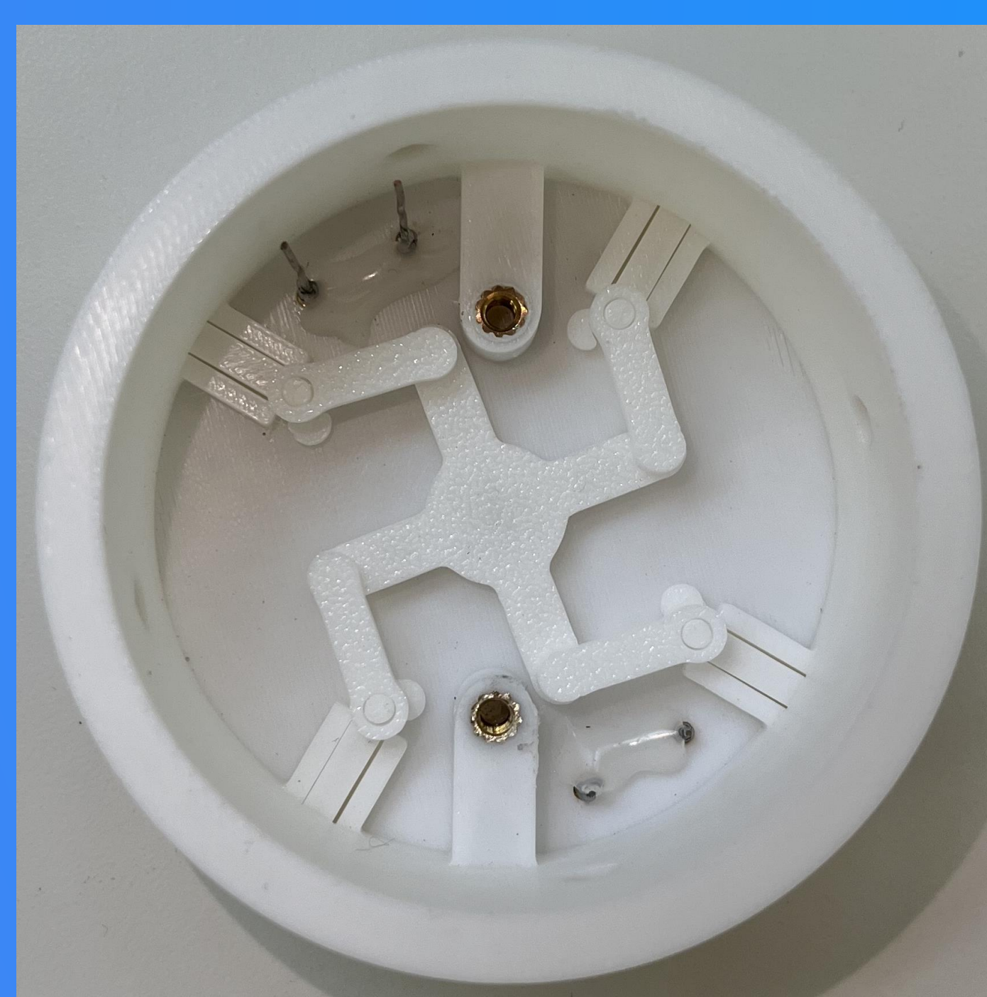
Newly designed tool changing mechanism
