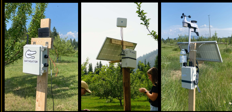
Figure 2: Left to right: Datagator, Gateway, WeatherRack Station
