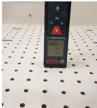
**Figure 3.8 Laser Distance Measuring Tool**
