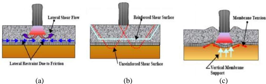
**Figure 2.8 Reinforcing effect of Geogrid (a) Lateral resistance; (b) Increased bearing capacity; and (c) Membrane effect (Holtz et al. 1998)**
