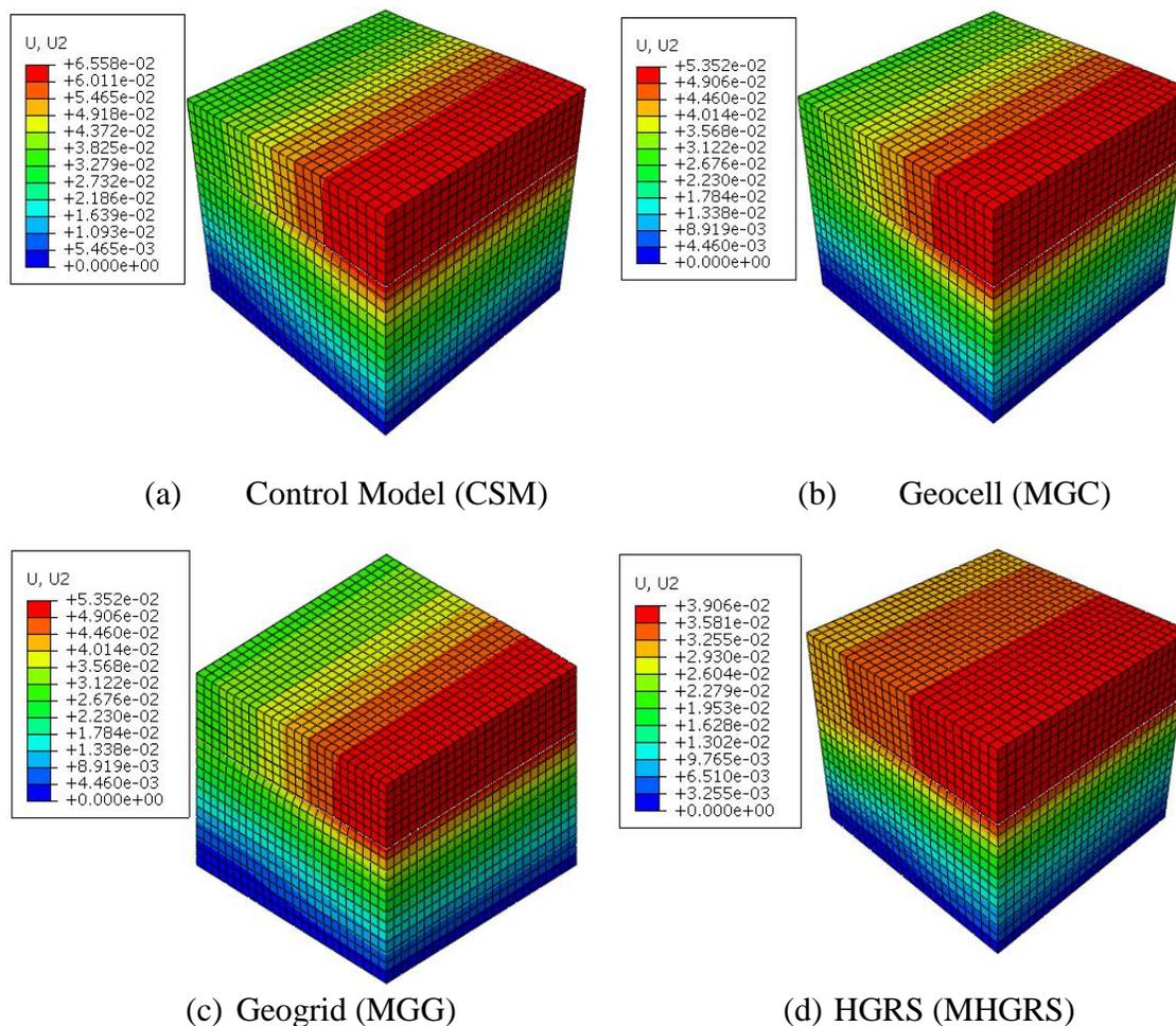
**Figure 4.26 Displacement Contours for the Numerical Models**
