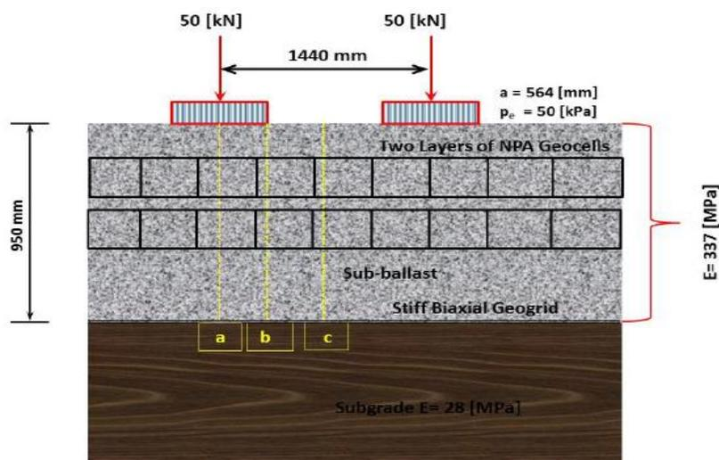
**Figure 2.12** Cross Section of Hybrid Geosynthetic Solution (Kief 2015)
