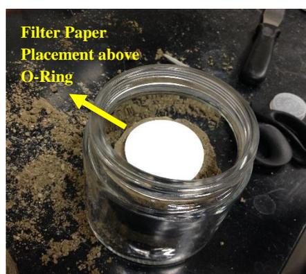
**Figure 4.4 Soil Specimen Prepared for Total Suction Measurement**
