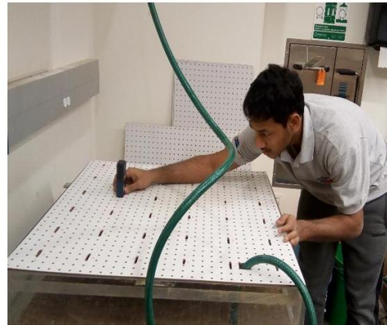
**Figure 3.18 Measurement of Vertical Swelling**
