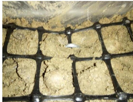
**Figure 3.25** Anchoring Geogrid using Steel Peg
