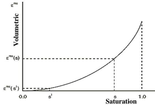
**Figure 4.6 Typical Volumetric Swelling vs Saturation Curve of Porous Medium (Dassault Systemes 2017)**
