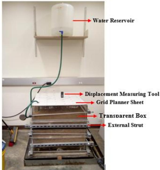
**Figure 3.9 Complete Set-up of the Large-Scale Box System**
