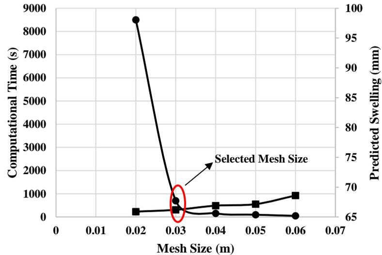
**Figure 4.11 Convergence Study to Optimize Mesh Size**
