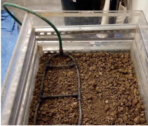
**Figure 3.15 Placement of Soaker System at the Top Half of Subgrade**
