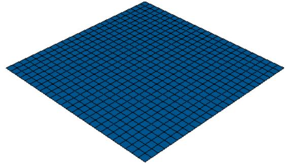
**Figure 4.21 Meshing Approach of Geogrid Sheet**
