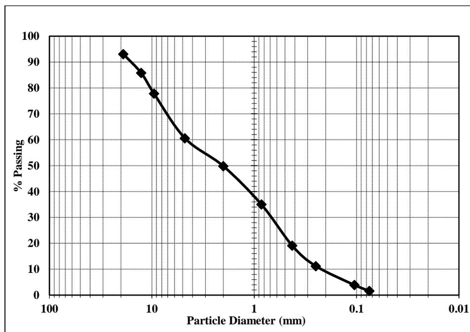
Figure B-4 Gradation Plot for Base Course Material
