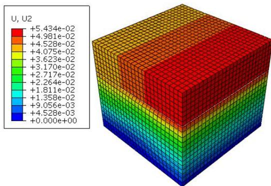
**Figure 4.30 Vertical Deformation Contour of HGRS for ES-2**
