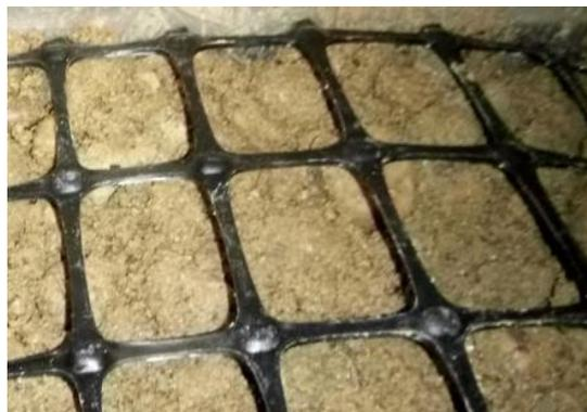
**Figure 3.11 Biaxial Geogrid Sample**
