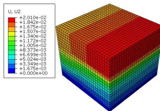
**Figure 4.31 Vertical Deformation Contour of HGRS ES-3**
