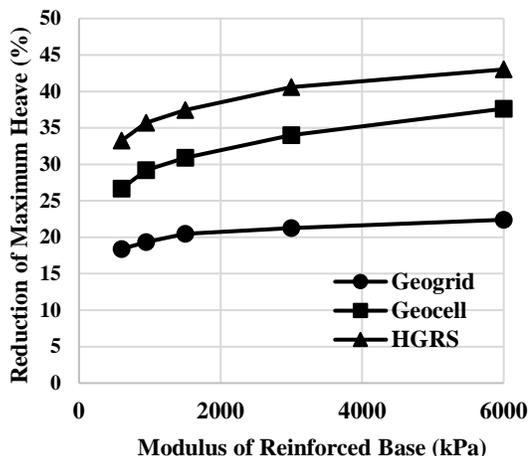
**Figure 4.34 % Reduction of Maximum Heave for Reinforced Base Layer with varying Modulus**
