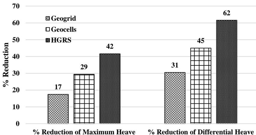
**Figure 3.30 Comparisons of Percent Swell Reductions for the Three Reinforced Test Sections**
