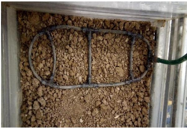
**Figure 3.4** Soaker System Arrangement
