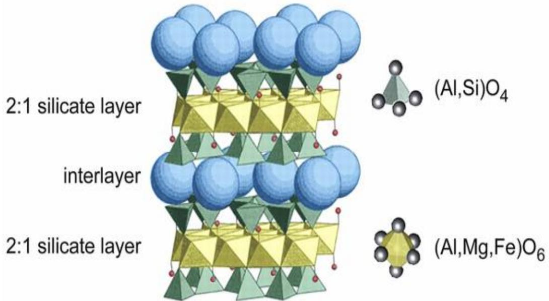
**Figure 2.1 Illustration of Montmorillonite Structure (Heyer 2012)**
