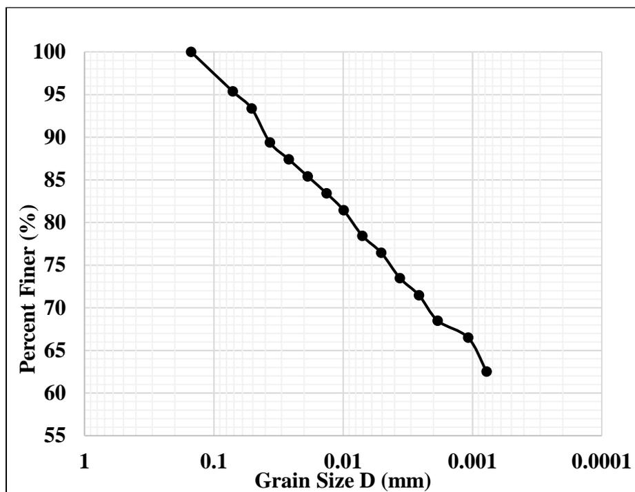
Figure B-2 Hydrometer Analysis Results of ES-1
