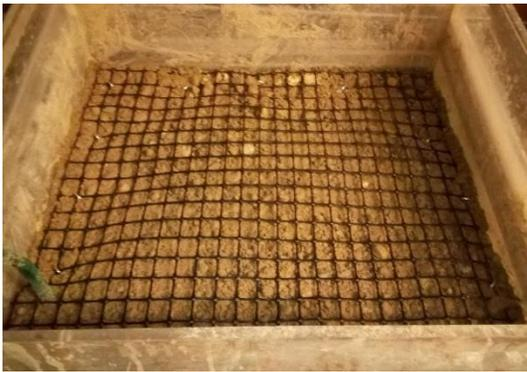
**Figure 3.27 Geogrid Installation in HGRS Section**
