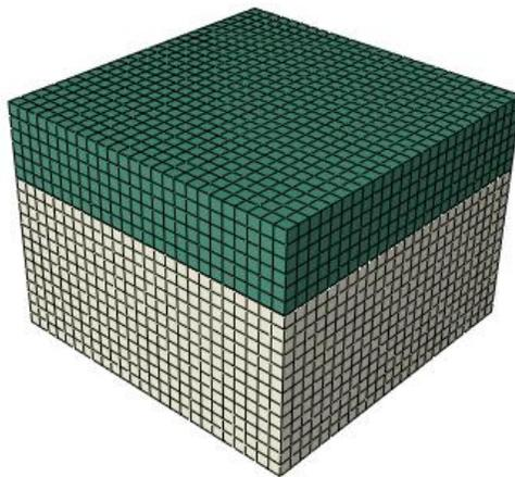
**Figure 4.12 Meshing of the CSM Model Section**
