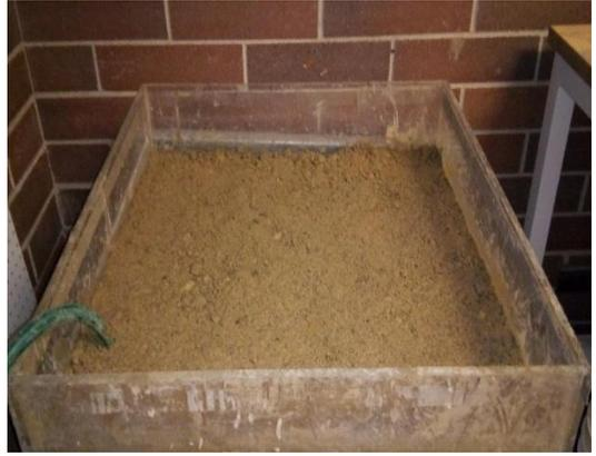
**Figure 3.21 GC Section after Compaction**
