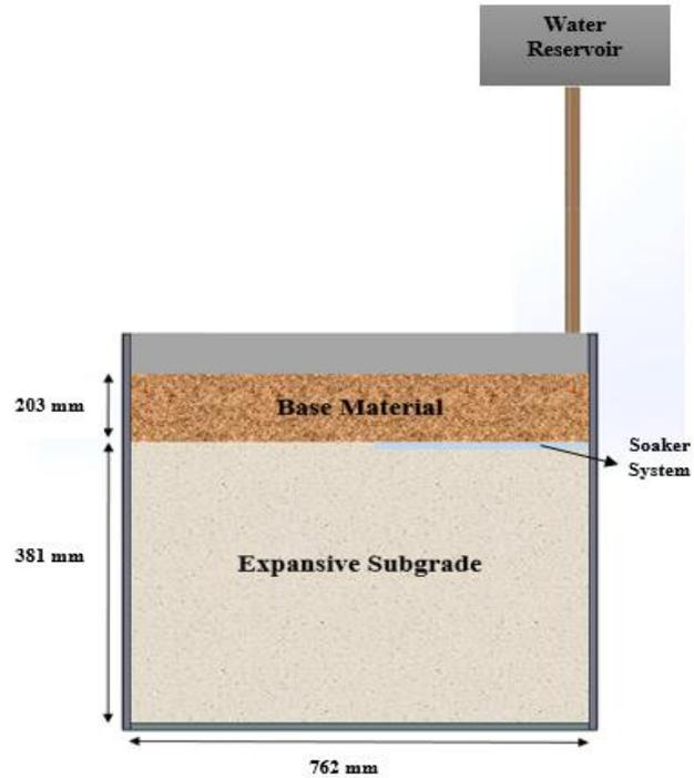
**Figure 3.1 Detail Schematic of Large-Scale Box System**
