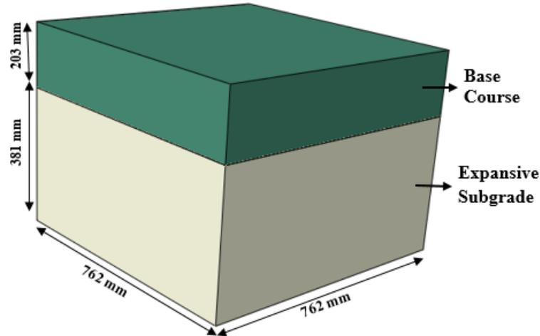
**Figure 4.1** Geometry of the Control Section Model (CSM)
