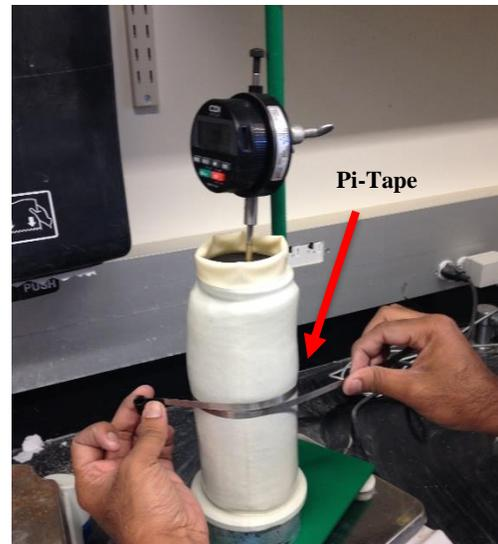
**Figure 4.8 Measurement of Radial Swell using Pi-Tape**
