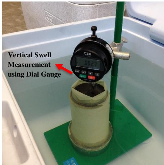
**Figure 4.7 Inundation of Soil Sample in Water Bath**
