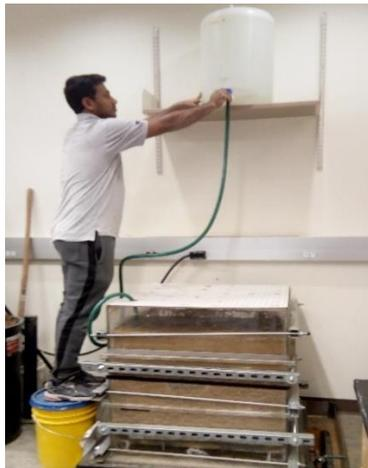
**Figure 3.17 Moisture Supply through Water Reservoir**
