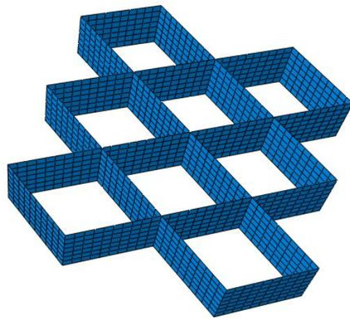
**Figure 4.17 Meshing Approach of Geocell**
