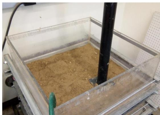
**Figure 3.14 Hand Compaction Tool**
