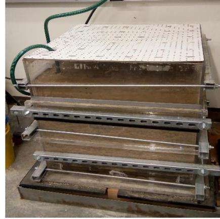
**Figure 3.16 Control Section after Compaction**
