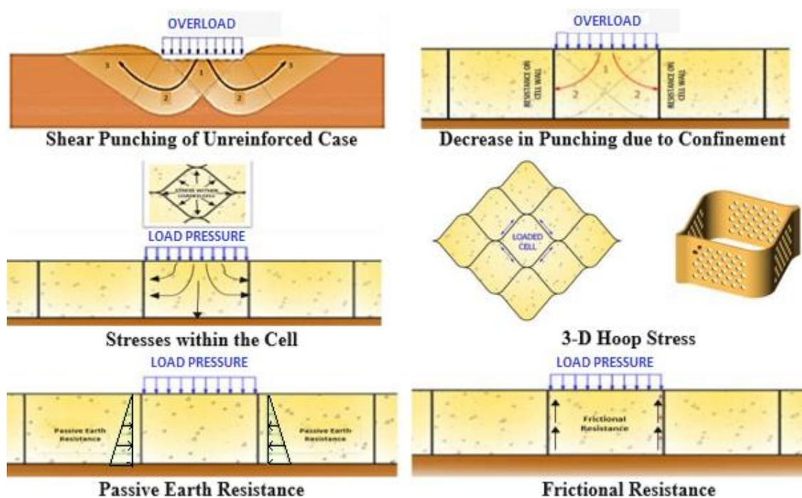
**Figure 2.6 Reinforcing Mechanism of Geocells (Tsorani 2008)**
