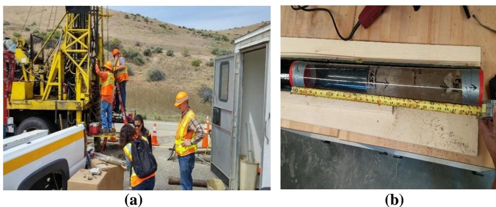
**Figure 3.6 Drilling and Sample Collections: (a) Full view of Drilling Operation (b) Plastic Tube Sampler with Soil Sample Inside (Sample Collected in May 2015; Courtesy-ITD)**
