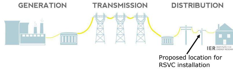
**Figure 7.1: Proposed location for the RSVC installation for CVR.**
