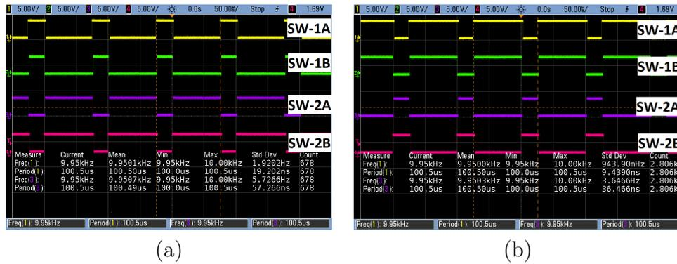
Figure 6.3: (a) IGBT gate driving signals at  $D = 0.25$  (b) IGBT gate driving signals at  $D = 0.75$ .
