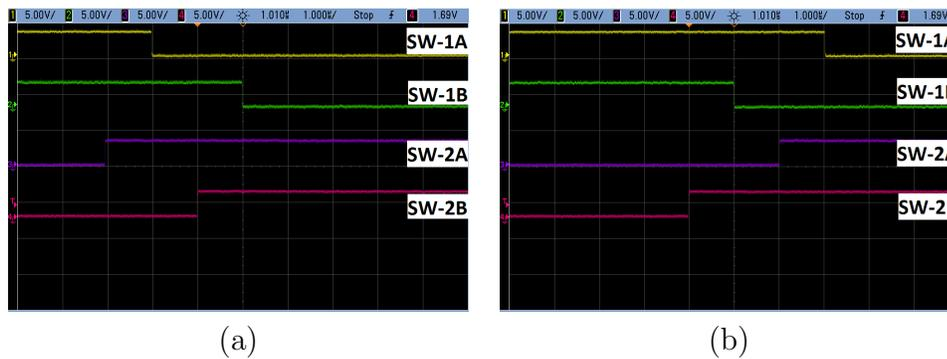
Figure 6.4: (a) IGBT gate driving signals transition from top switch to bottom switch when input voltage is greater than 0 ( $V_{SVC} > 0$ ) (b) IGBT gate driving signals transition from top switch to bottom switch when input voltage is less than 0 ( $V_{SVC} < 0$ ).
