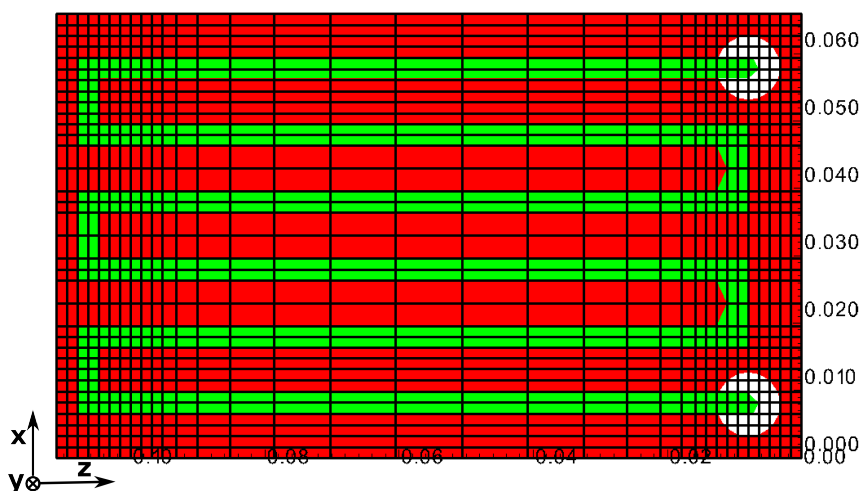
Figure 5.13: Vsim non-uniform mesh on the X-Z plane. The green section is the meander line, red is the ground plane, The white circles are the space between the inner and outer conductor of the coaxial cable, and the black lines are the mesh. In X, regions which coincide with the circuit is 2 cells wide and regions between the circuit is 2 cells wide. In Z, the circuit region is 2 cells wide, but in the center, the length of the cells is increased.
