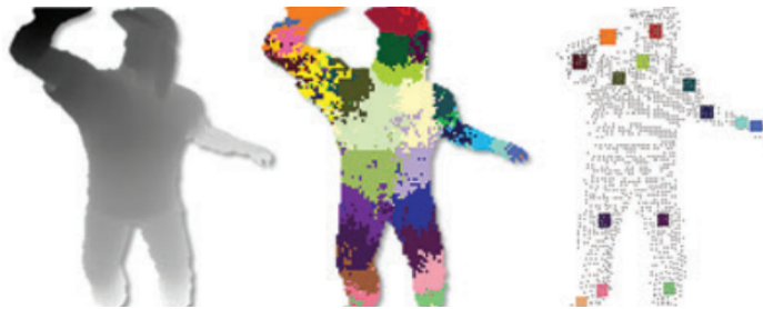
Figure 2.8: Body joint estimation procedure.
