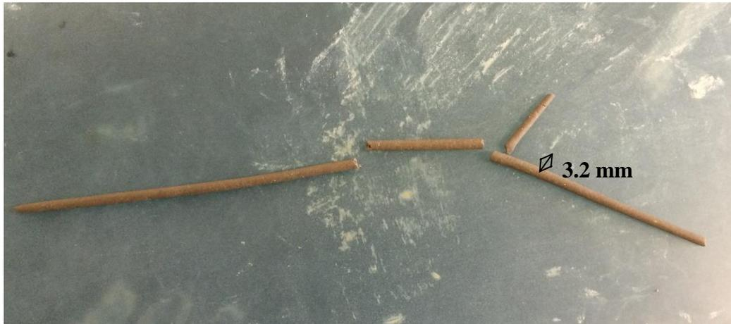
**Figure 8.**      **Plastic limit test.**
