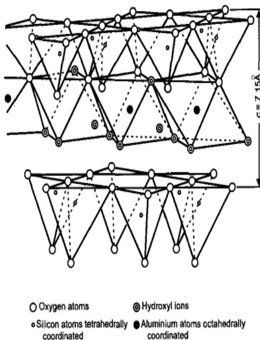
**Figure 2. Schematic of the structures of Kaolin (Murray, 1999)**
