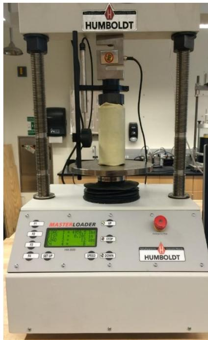
**Figure 13. UCS test setup used in this research**
