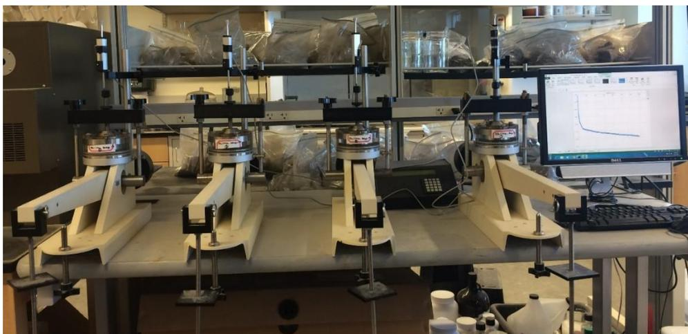
**Figure 14. 1-Dimensional swell test**
