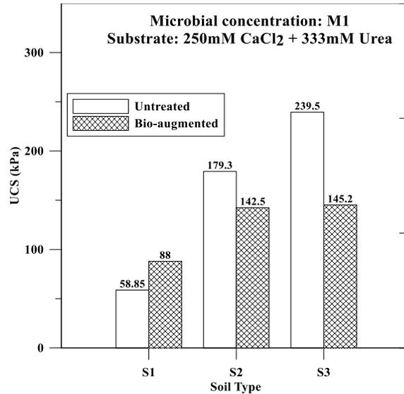
**Figure 18. UCS values of untreated and bio-augmented soil samples**
