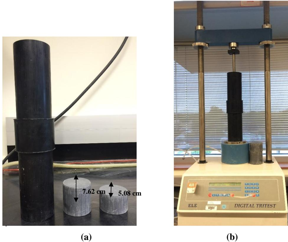
**Figure 12. (a) Tube and blocks used for sample preparation (b) static compactor used for sample compaction**
